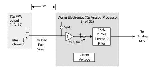
Figure 7. MIPS Ge FPA Analog Chain Block Diagram
