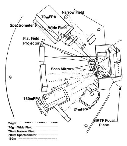
Fig. 4 MIPS Optical Layout
