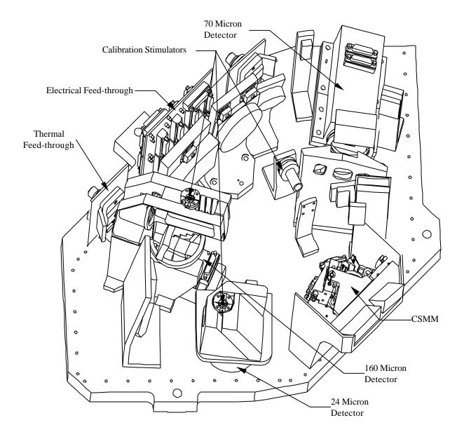
Figure 1. The MIPS Cold Instrument Assembly.
