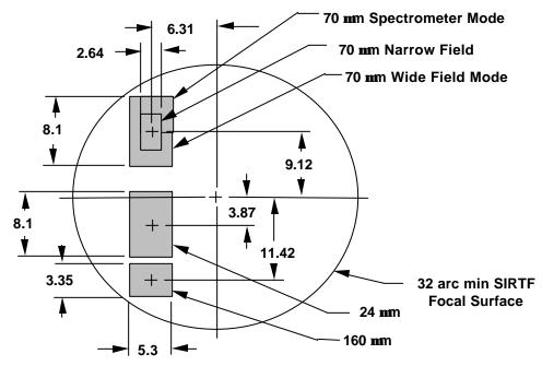
Fig. 3 MIPS Fields of View in the SIRTF Focal Surface
