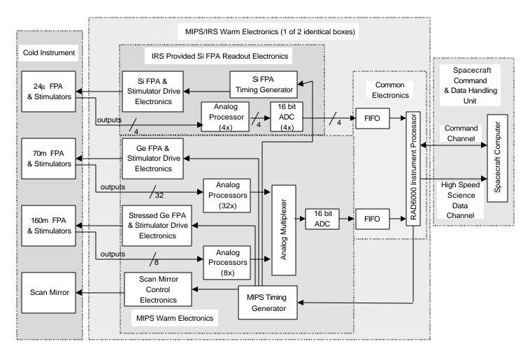
Figure 6. MIPS Electronics Block Diagram
