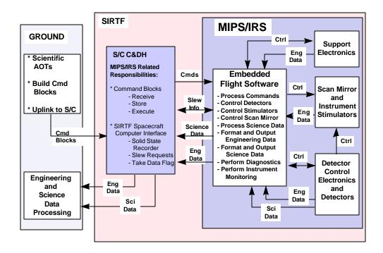
Figure 8. MIPS Software Block Diagram
