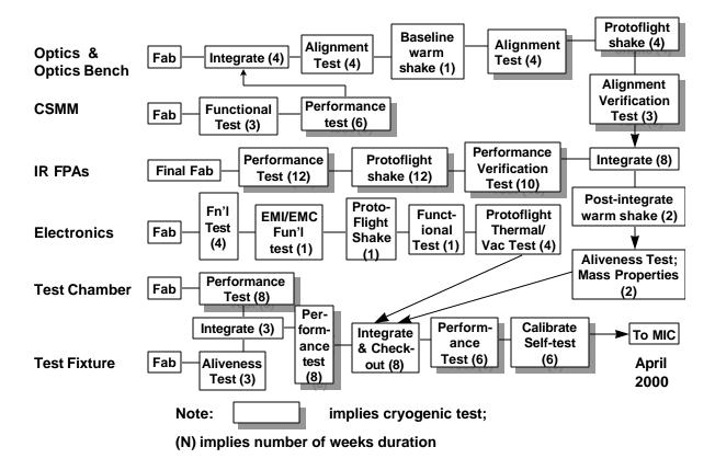
Figure 9. MIPS Integration and Test Flow Diagram
