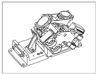
Figure 2. MIPS Cryogenic Scan Mirror Mechanism.
