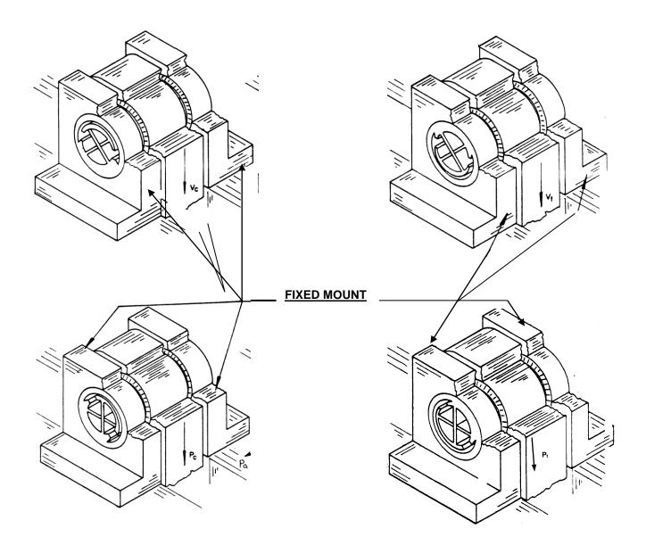
WHERE A Pt OR Vt CONDITION EXISTS A Pc OR Vc CONDITION MAY BE OBTAINED BY ROTATING THE PIVOT 180 DEGREES OR CONVERSELY A Pt OR Vt MAY BE OBTAINED FROM A Pc OR Vc LOADING BY ROTATING THE PIVOT 180 DEGREES WITHIN FIXED MOUNT.
